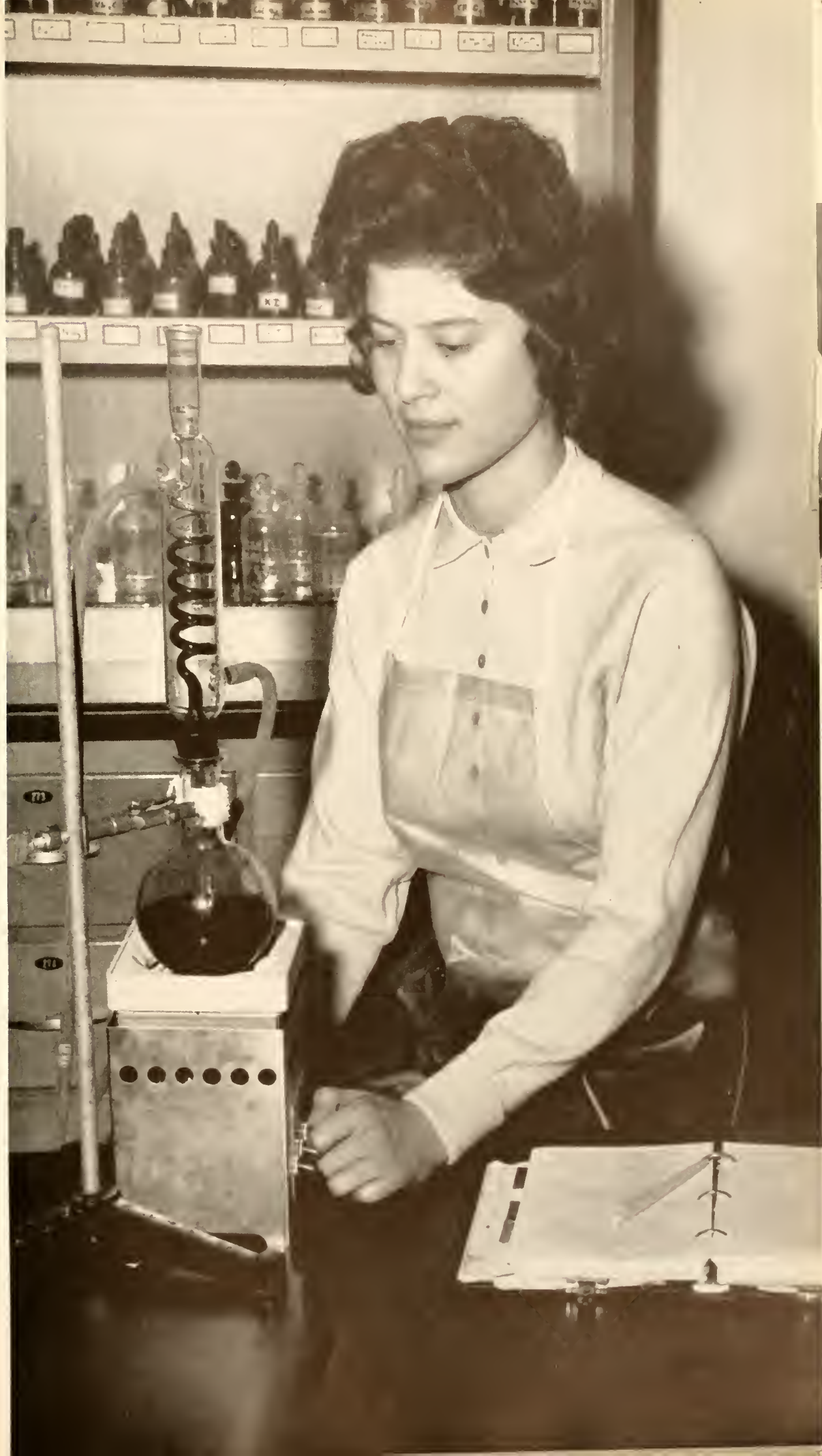
Attempting an experiment in organic chemistry, Sally Franklin prepares a complex carbon compound with a reflux condenser.
